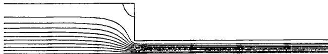
Figure 27. Streamline plot for the flow of a Newtonian fluid in a 4:1 symmetric sudden contraction ( Re = 10 , Pe = 100 , Br = 1 , A = 0.1 ) (Example 5)
